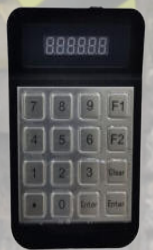
DUR087066: Height adjusting keypad for low bridge detection system.
